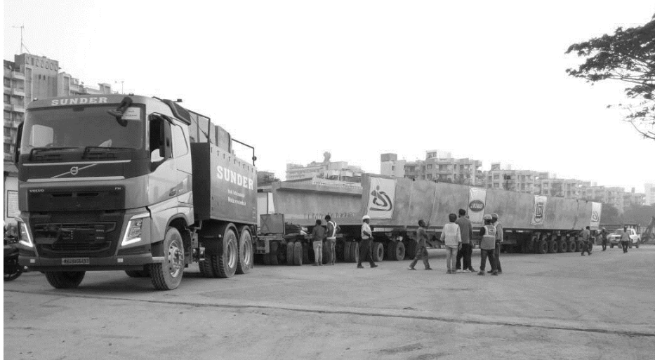
Figure 14 Transportation of Full Span U Girder: Mumbai Line 7
